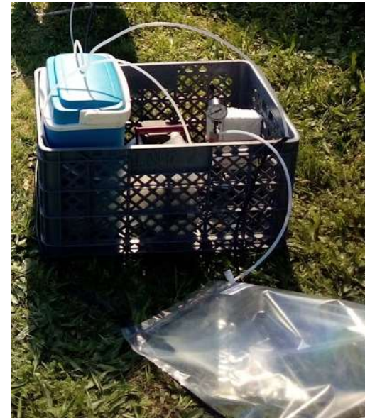
Water condensation unit, flowmeter, pump and Tedlar bag
